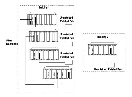
Figure 2-3. Star-Wiring Configuration
